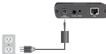
FIGURE QS-7. CONNECT THE REMOTE EXTENDER TO THE AC ADAPTER AND A POWER SOURCE
