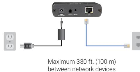
FIGURE QS-3. CONNECT THE REMOTE EXTENDER TO A NETWORK SWITCH
